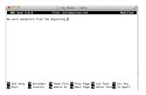
In nano, use Control-X to quit the editor and return to the shell. Make sure you save in the process. We can check the changes we've made to a particular file by using the *cat* command.
